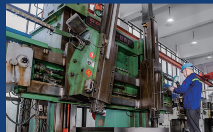
2.5-meter Vertical Lathe
